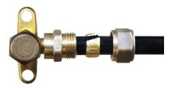
8. Screw on the connector nut by hand, again using a torque spanner to tighten the connector nut to the recommended torque<sup>3</sup>. Remember to hold the union in place. It is recommended to fix the union with a threadlocker. (Loctite 242 or Loctite 243).
