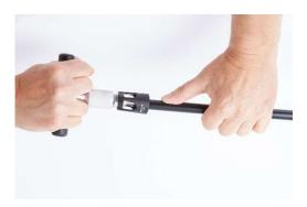
5. Screw the UFLEX® adapter fitting onto the unit valve of the air conditioner (condensor / compressor). We recommend the use of an appropriate copper seal and threadlocker (Loctite 242 or Loctite 243).
